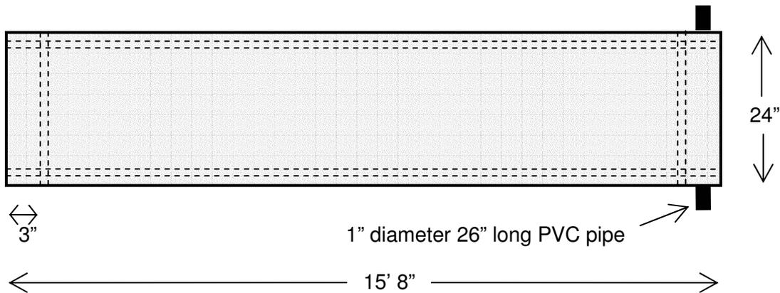
\*Note. For illustrative purposes, only one PVC pipe is shown. When in use, PVC pipes are put in both the top and bottom pockets on the banner.
